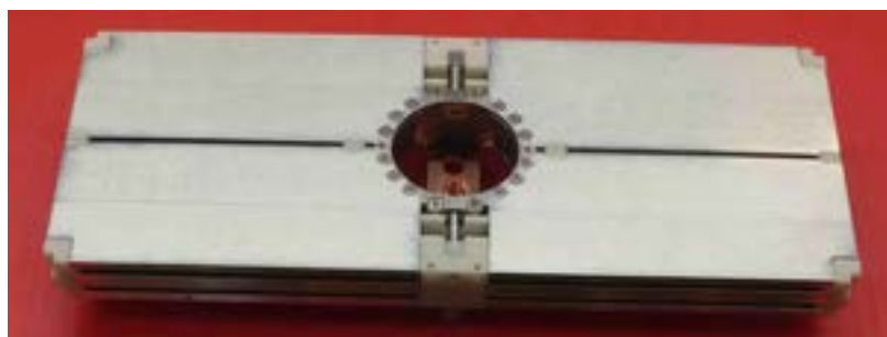
Figure 7. Flight capacitor bank with 1232 MLCC capacitors storing a total of \sim 31.5 J of energy.
