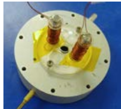
Figure 18. Assembled unit with electromagnets installed.
