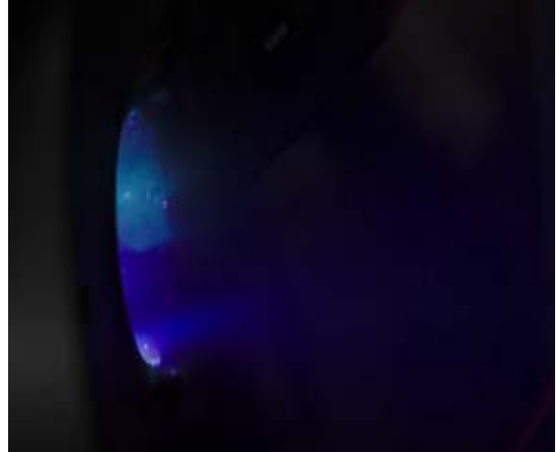
Figure 24. Thruster firing with electromagnets turned on with current flow in the “reverse” direction. Camera is looking down from above.
