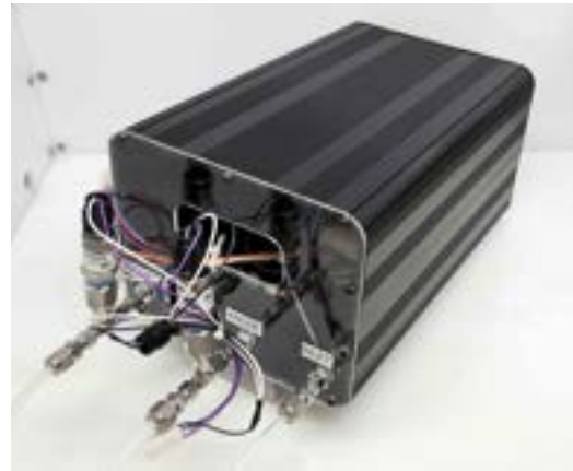
Figure 3. Breadboard CAMFlow-1 system with additional pressure sensor monitoring.
