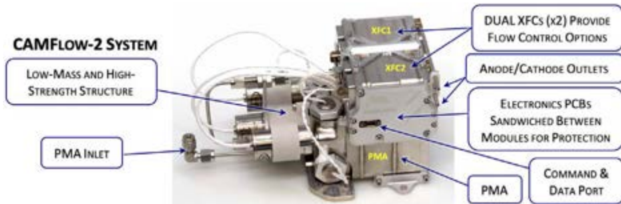
Figure 22. The CAMFlow-2 system with mass of 2.2 kg consists of multiple modular sections: (1) the Pressure Management Assembly (PMA) accepts up to 2,500 psia of input pressure; (2) the primary Xenon Flow Controller (XFC) controls the output flow rate to < \pm 3\% ; and (3) a secondary, optional XFC provides an initial boost to the cathode flow leg and allows operation with heaterless cathodes.
