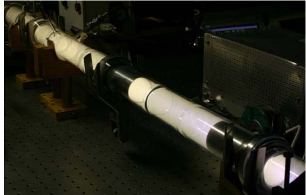
Figure 3: Photograph of ElectricOIL flow tube with active discharge using hollow electrodes.
