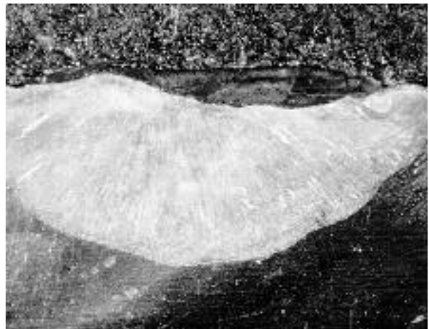
Fig. 9 Cross sectional view of the ceramic clad, clad-substrate interface and substrate melt pool. Magnification: 18. Cladding mixture: 95.08% ZrO 2 and 4.92% Al by wt. Substrate: Stainless steel. Laser parameters: Incident power = 4.65 kW, Scanning speed = 0.5 cm/s, 4mm x 1mm rectangular spot.
