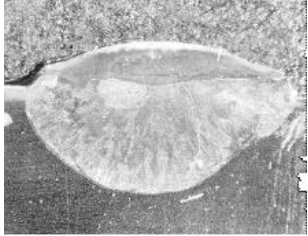
Fig. 11 Cross sectional view of the ceramic clad, clad-substrate interface and substrate melt pool. Magnification: 18. Cladding mixture: 80.04% ZrO_2 and 19.96% Al by wt. Substrate: Stainless steel. Laser parameters: Incident power = 4.72 kW, Scanning speed = 0.5 cm/s, 4mm x 1mm rectangular spot.
