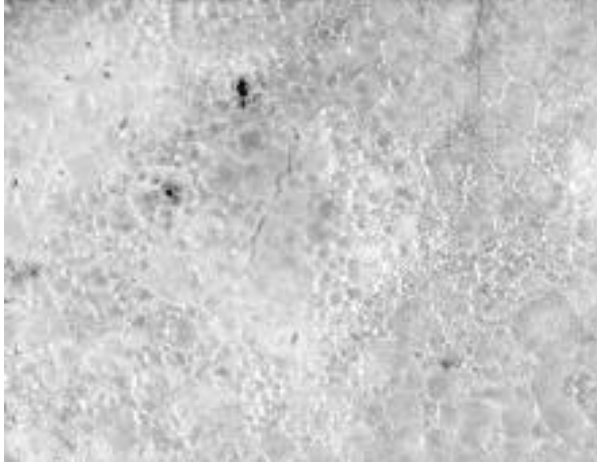
Fig. 10 Surface morphology of a laser ceramic clad. Magnification: 35. Cladding mixture: 80.04% ZrO_2 and 19.96% Al by wt. Substrate: Stainless steel. Laser parameters: Incident power = 4.72 kW, Scanning speed = 0.5 cm/s, 4mm x 1mm rectangular spot.
